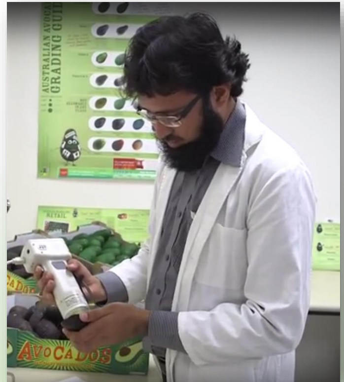
Using a colour meter to measure bruise intensity
