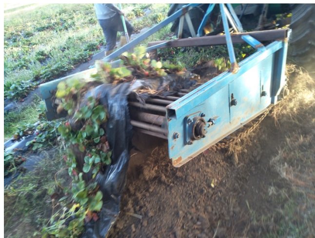
Modified garlic digger lifting plastic and plants, including the crowns (Photo credit: Portland Strawberries)
