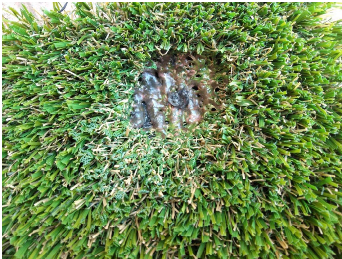
Figure 2 Example of melted synthetic turf from point ignition source
