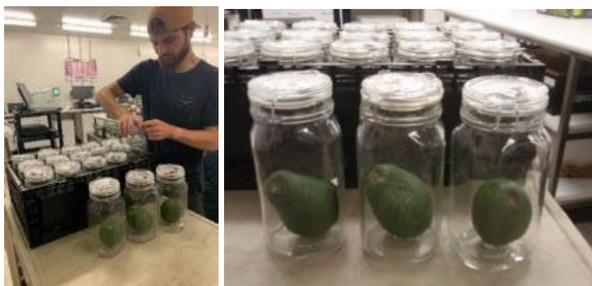
Figure 1. Measurement of headspace \text{CO}_2 and ethylene produced by Hass avocado in sealed glass jars to measure fruit respiration and ethylene production rates.
