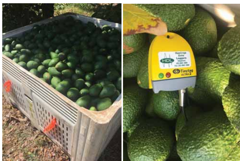
Figure 3. A marked bin (left) and data logger with probe used to monitor temperatures of fruit inside (right).
