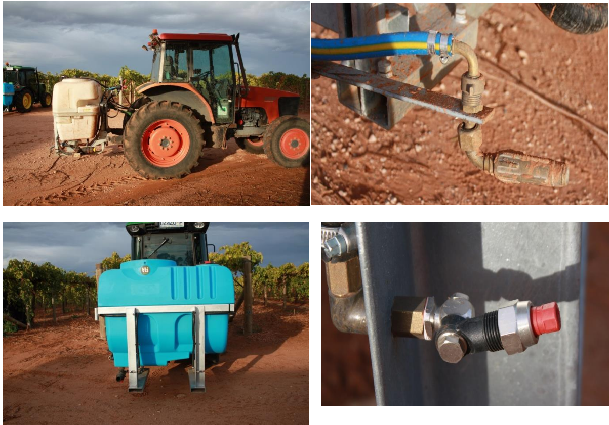
Figure 11: Three point linkage mounted sprayers (left) and close up of the jets (right).
